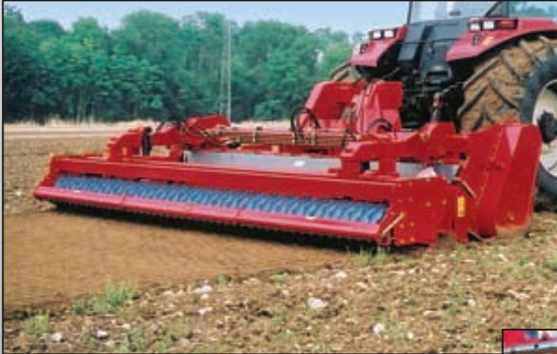
RXX 400 Super heavy duty Soil Renovator™ for large areas : golf courses construction, sod farms, pastures renovation...
