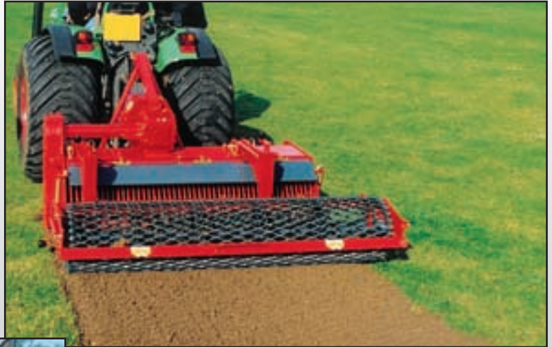
Direct operation with the RD 150 compact Soil Renovator™.
