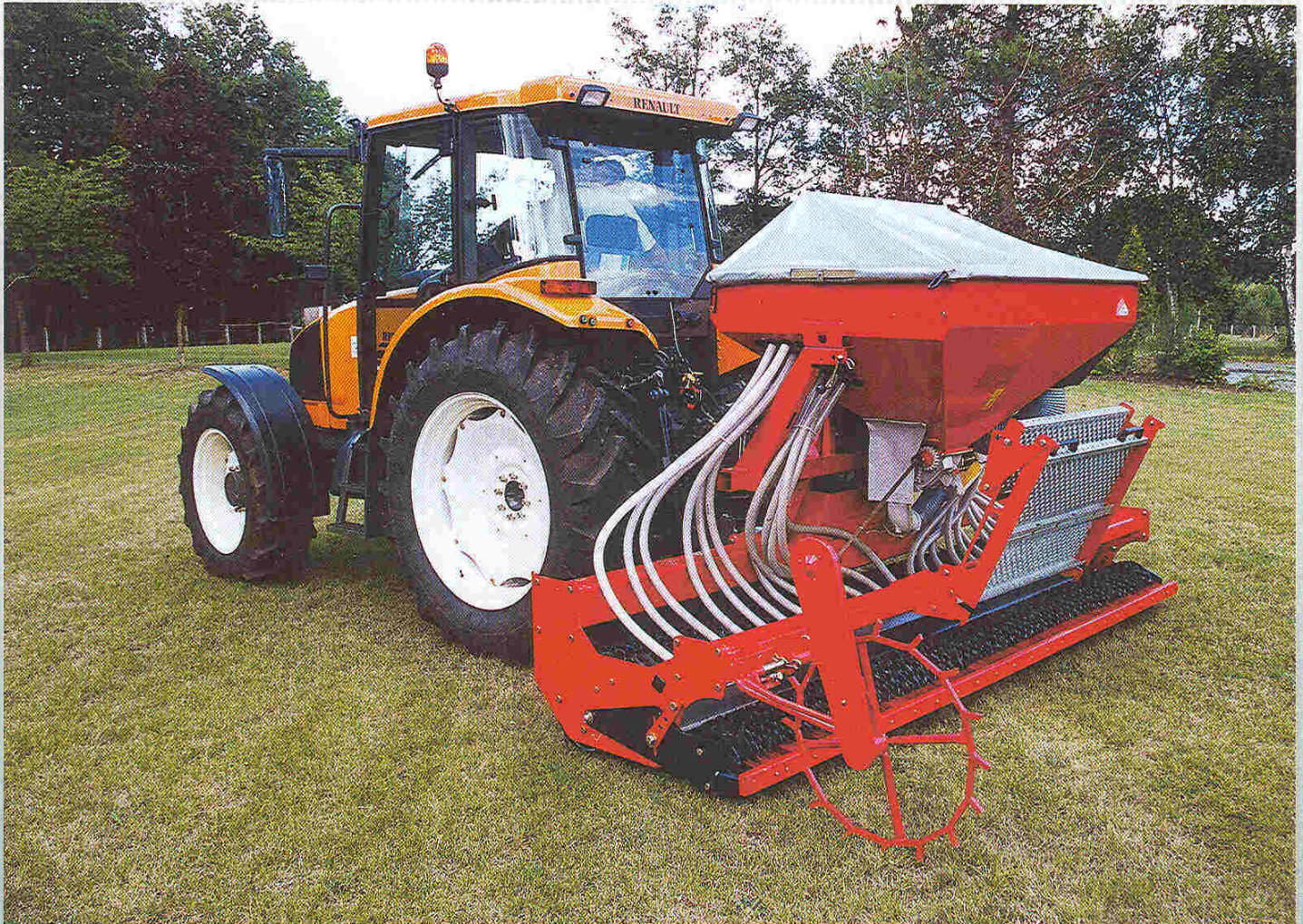
SMA 305 Primary Pneumatic Seeder notched rollers
